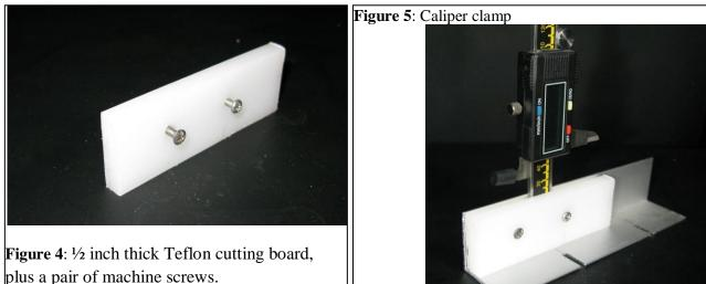
I used 6:32 screws and tapped the holes in the angle aluminum - - you could just as well use a pair of 6:32 nuts here. Note the hole slots in the angle aluminum and the vice clamp nature of the of the caliper attachment allow two degrees movement freedom for alignment of the caliper with the movable scope optics.
