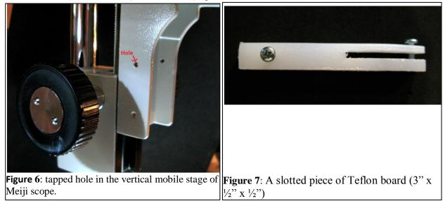
A machine screw was inserted across the lower end of the slot to function as a squeeze vice. A hole was drilled in the upper end of the piece for my metric screw attachment to the scope, (Figure 8). Assembling all the pieces together provides the configuration illustrated in figure 9.
